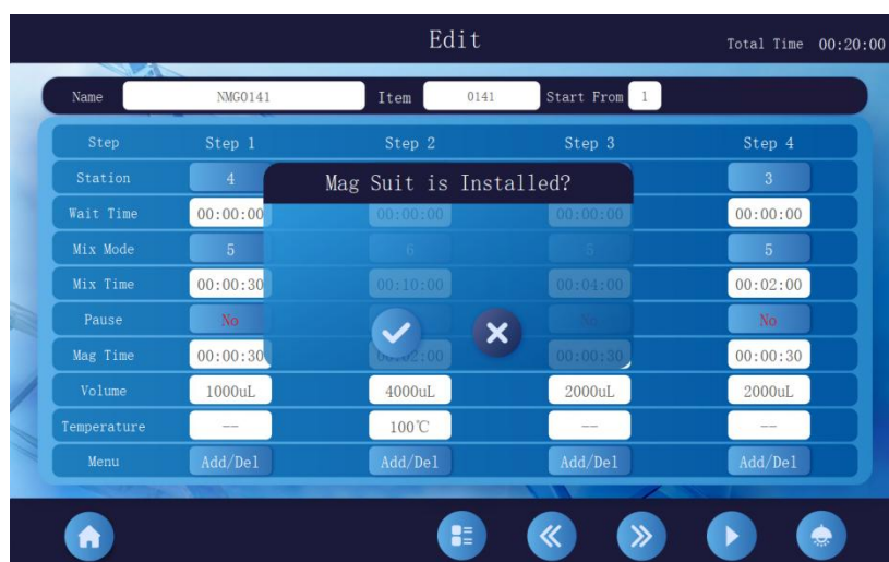
Figure 9: Magnetic Sheath Installation Prompt
